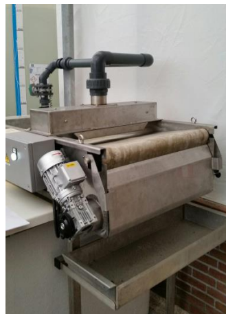
Figure 3-11. Paper band filter (source FERTINNOWA)
